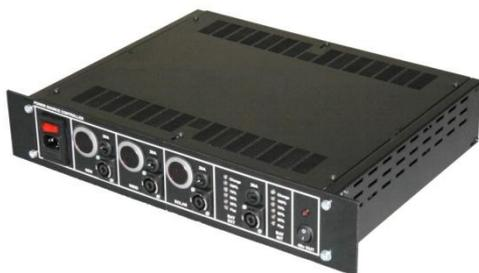
19" Rack, Six Channel PSC with Displays and Mains Input PSU
