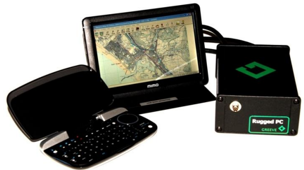
Platform PC with 7" screen and remote micro keyboard
